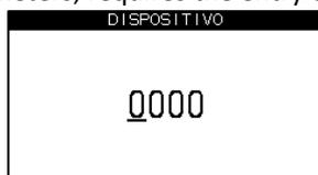
Enter one digit at a time; use the LEFT\_BUTTON and RIGHT\_BUTTON to move the cursor, and the UP\_BUTTON and DOWN\_BUTTON to change the digit. To test, use the CONFIRM\_BUTTON until the result appears:
