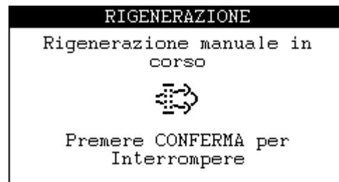
You can follow the status of the manual regeneration through the signals in the instrument LAMPS.
