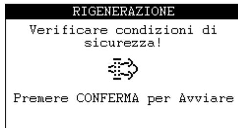
In both cases the operator will be requested to start the procedure by pressing and holding the CONFIRM\_BUTTON for around 3 seconds.
