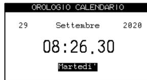
The value shown can be changed using the UP\_BUTTON or DOWN\_BUTTON. To change selection, use the RIGHT\_BUTTON or the LEFT\_BUTTON. To exit settings, press the PUMP\_PROTECTIONS\_DISABLE\_BUTTON. It does not require confirmation. The time is retained by the control unit even when it is not powered, thanks to an internal battery.
